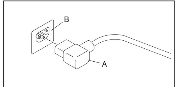
2. Plug the power cord (A) into an appropriate outlet (C) that is properly installed and earthed in accordance with all local codes and ordinances.
