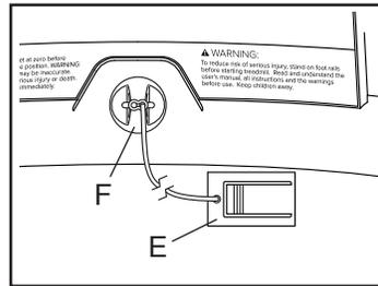
insert the key into the console. **Note: It may take some time for the console to be ready for use. IMPORTANT: In an emergency, the key can be pulled from the console, causing the walking belt to slow to a stop. Test the clip by carefully taking a few steps backward; if the key is not pulled from the console, adjust the position of the clip.**
