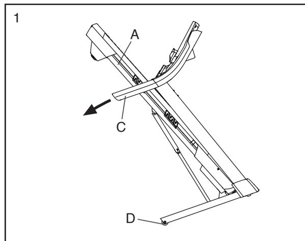
2. Pull back on the handrail until the treadmill will roll on the wheels, and carefully move it to the desired location. **CAUTION: Do not move the treadmill without tipping it back, do not pull on the frame, and do not move the treadmill over an uneven surface.**
