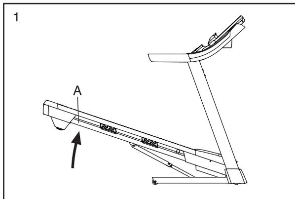
2. Raise the frame (A) until the storage latch (B) locks in the storage position. **CAUTION: Make sure that the storage latch locks.**
