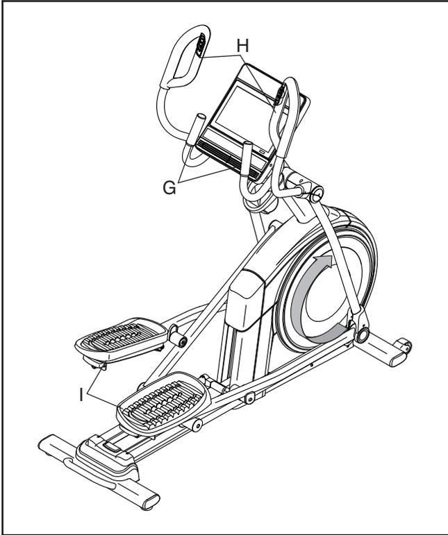
To dismount the elliptical, wait until the pedals (I) come to a complete stop. **Note: The elliptical does not have a free wheel; the pedals will continue to move until the flywheel stops.** When the pedals are stationary, step off the higher pedal first. Then, step off the lower pedal.
